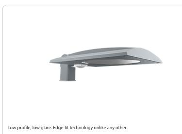
**Project:** Type: Prepared By: Date: **LED Info Driver Info Constant Current** Watts 94W Туре 120V 0.83A Color Temp 4000K (Neutral) 208V 0.48A Color Accuracy 72 CRI 240V 0.42A L70 Lifespan 100,000 Hours
