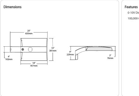
0-10V Dimming, standard 100,000-Hour LED lifespan
