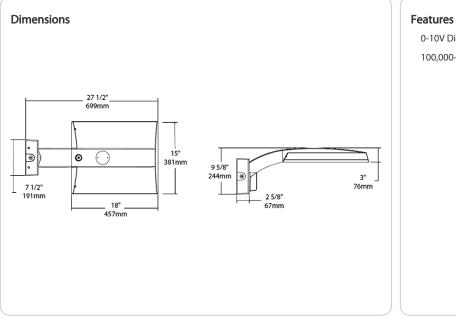
0-10V Dimming, standard 100,000-Hour LED lifespan
