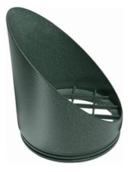
Die cast aluminum visor with integral metal grill and tempered glass lens for maximum glare reduction and lamp protection. Guard protects lamp from damage and vandalism. Die cast aluminum.
