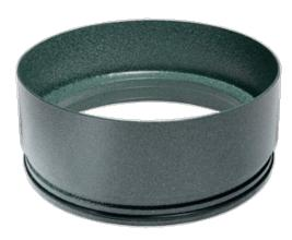
Hood with tempered glass lens reduces glare and protects lamp from water and impact damage. Die cast aluminum. Fits H101 and HB101. Can be combined with HG1 Guard.
