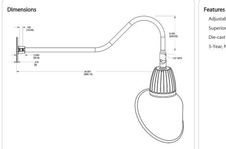
Adjustable 45° swivel joint Superior heat sink Die-cast aluminum housing 5-Year, No-Compromise Warranty
