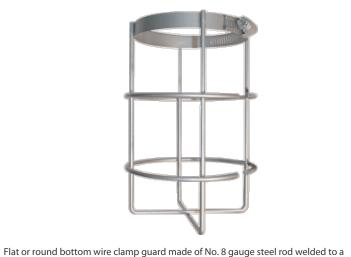
Flat or round bottom wire clamp guard made of No. 8 gauge steel rod welded to a clamping band. Guard is protected from corrosion by a baked silver gray polyester powder finish.
