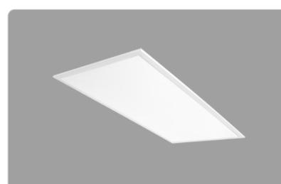
2' x 4' EZPANHE edgelit LED panel lights with emergency battery Backup that will operate the LED Lamp for 90 minutes if power fails. Install in drop ceilings or use optional surface, pendant or recessed (dry wall) mounting kits.
