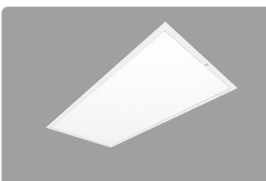
2' x 4' EZPAN edgelit LED panel lights with emergency battery Backup that will operate the LED Lamp for 90 minutes if power fails. Install in drop ceilings or use optional surface, pendant or recessed (dry wall) mounting kits.
