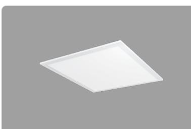
$2' \times 2'$  EZPAN edgelit LED panel lights with emergency battery Backup that will operate the LED Lamp for 90 minutes if power fails. For use in drop ceilings or drywall using the optional recessed mounting kit.
