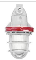
Explosionproof fixture for ceiling mounting. Set screw to stern prevents rotation. Cast aluminum housing, heat and impact resistant globe. Fits all incandescent lamps up to 300 Watt PS-25. Lamp not supplied.
