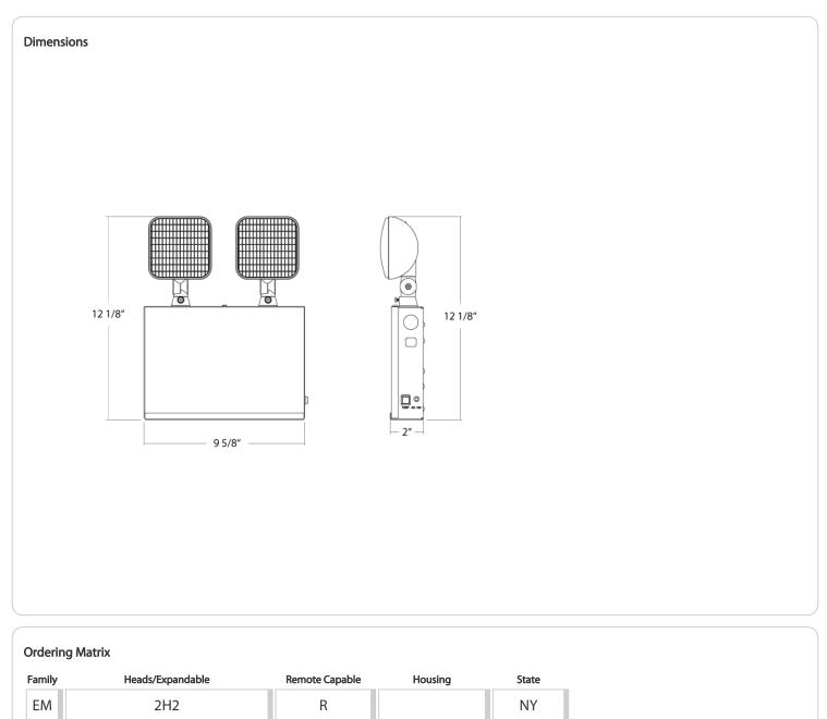
2H2 = 2 Heads Integral/Expandable 2 HeadsR = Remote CapableBlank = White HousingNY = New York2H6 = 2 Heads Integral/Expandable 6 Heads
