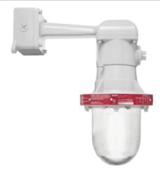
Explosion proof fixture for wall mounting. Cast aluminum housing, heat and impact resistant globe. Fits all incandescent lamps up to 300 Watt PS-25. Lamp not supplied.
