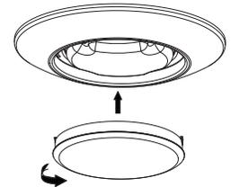
6. Screw the E26 adapter into the socket. Then connect male connector of E26 adapter to the female connector of the disk (Fig.23) Simply slide the trim and torsion springs into the housing. (Fig.24) Carefully place wires into fixture and push the LED trim into the housing until flush with ceilings. (Fig.25)
