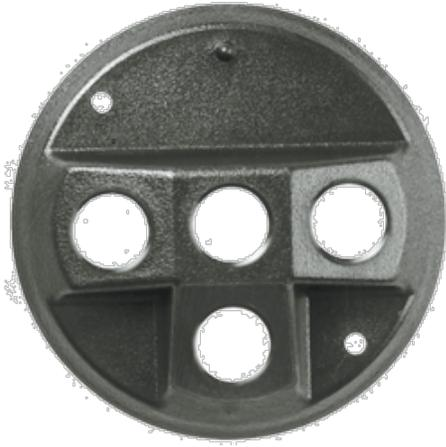
Corrosion-proof round four hole cover. Tough polycarbonate with molded-in color. Fourth hole is perfect for motion sensor mounting. Fits 4" round boxes. Supplied with thick foam rubber gasket. One molded 1/2" close-up plug and (2) stainless steel screws.
