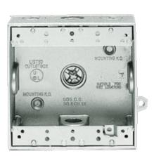
Die cast aluminum with two unique "flex-lugs" for wall or pole mounting of outdoor outlets, switches or floodlights. Ground screw and close-up plugs provided. Cubic capacity is 30.5 cu. inches.
