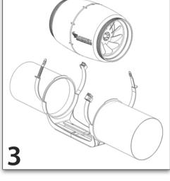
To install the S-line fan, the fan assembly must first be removed. To unlock the mounting bracket: while lifting the LIFT button (1), push the security tab (2) down and open the flange.
