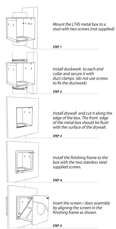
The Lint Trap should always be inspected and cleaned before the use of the dryer, as this will decrease drying times and help prevent any hazardous lint build-up.
