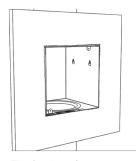
Install drywall and cut it along the edge of the box. The front edge of the metal box should be flush with the surface of the drywall.
