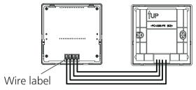
(11) Fix the wall control screen to the face plate backing cover. Upside snap joint —
