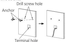
(9) Route the cables form the unit to the terminal hole.
