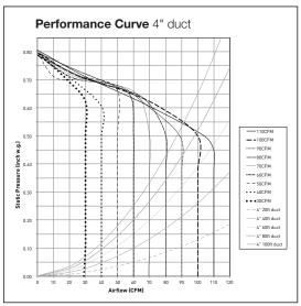
\*Industry research indicates static pressure in typical installations ranges from 0.20" to 0.375
