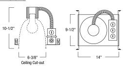
Cut-out: 6-3/8" ID: 6" Housing Length: 14" Housing Width: 9-1/2" Housing Height: 10-1/2"
