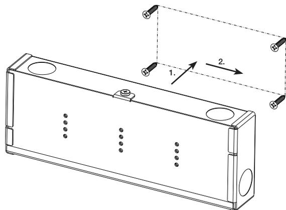
3. Open the necessary knockouts to pass wires into the wiring compartment.
