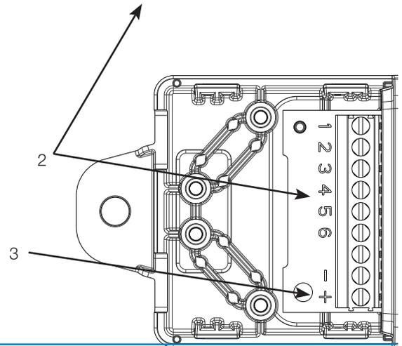
4. Install the strain relief and tighten the screws.
