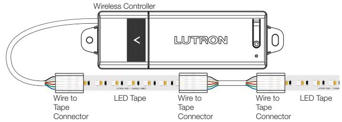
a. Measure and cut the length of cable needed to connect the tapes in their installed locations.
