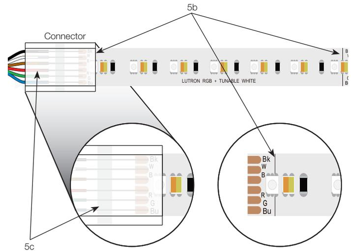
c. Insert **unstripped**, Lutron provided, 22 AWG (0.50 mm<sup>2</sup>) wires into the wire holes in the connector ensuring to align the wire color to the appropriate channel on the tape.
