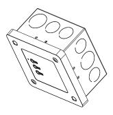
Note: 101.6 mm x 101.6 mm (4 in x 4 in) junction box not provided by Lutron. Shown here with fully installed product.
