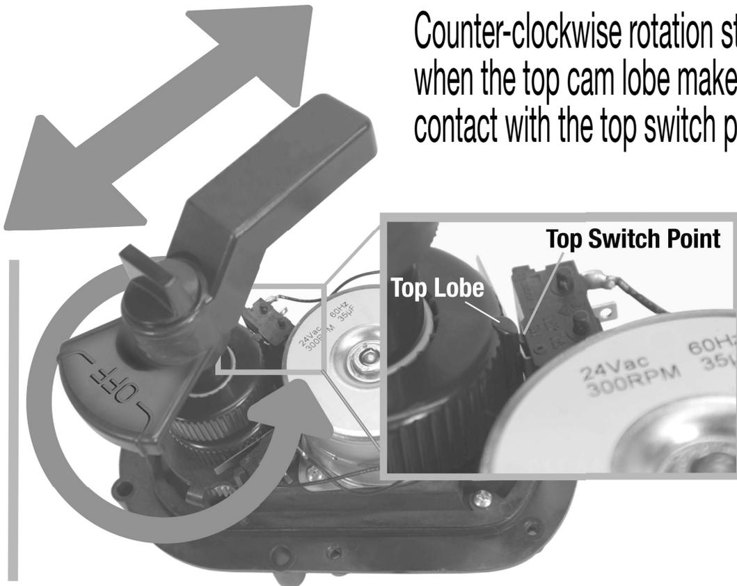
Counter-clockwise rotation stops when the top cam lobe makes contact with the top switch point.
