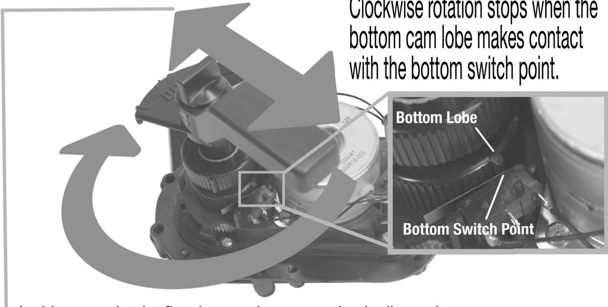
In this example, the flow has not been completely diverted at the stopping point.
