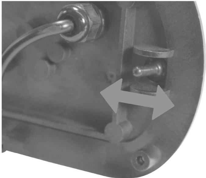
To check the clockwise stopping point, activate the bottom switch in the opposite direction.
