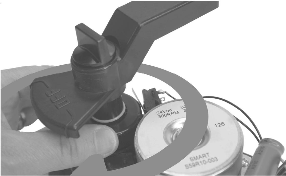
Push down and turn the top cam to change the position of the stopping point.
