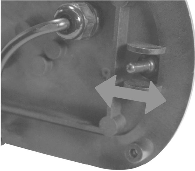
Test the position of the stopping point by toggling the bottom switch.
