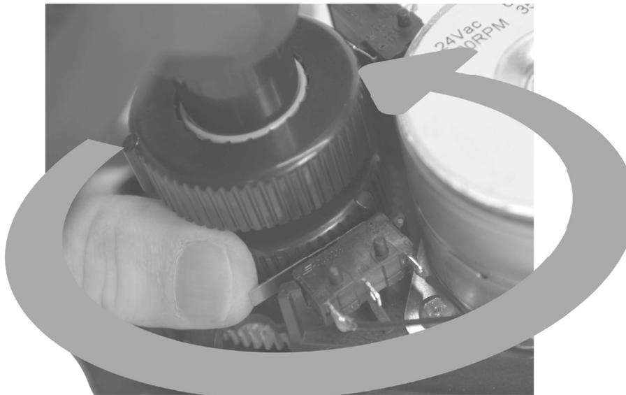
Push down and turn the bottom cam to change the position of the stopping point.
