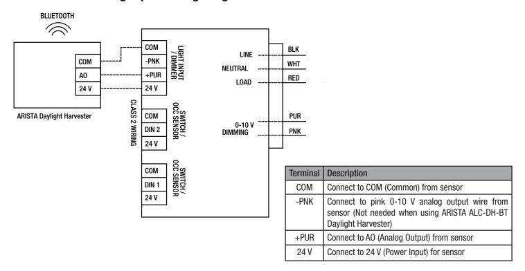
Note: 1. Maximum wiring distance <= 200' with a minimum size of 24 AWG; maximum size of 16 AWG.
