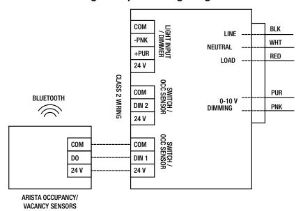
NOTE: Communications can be done through the Bluetooth Mesh network or be wired when using 24 VDC.
