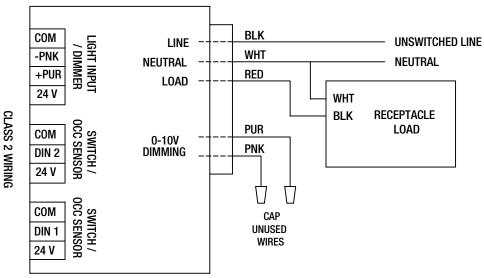
**NOTE:** When using the ALC1-R for plug load control, the purple and pink wires should be individually capped and will not be used.
